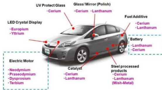
Figure 1. Critical elements used in various components of a modern motor vehicle Source: Universiteit Leiden
